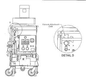
Normal surface preparation will usually be accomplished with the vacuum adjustment gate partially open. A period of trial and error may be necessary for specific job applications. Generally speaking, the more dust generated by your surface preparation equipment, the greater the suction you will need from the dust collector to keep the abrasive as clean as possible.
